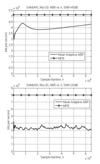
Figure 5 Ch. 3 Equalization by SAM, 45dB and 20dB
