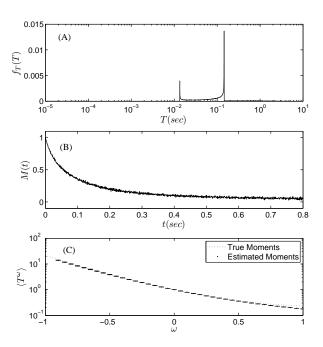
Figure 1: (A) A complex  $f_T(T)$  is considered. (B) Data simulated from this model with additive white Gaussian noise with  $\sigma_{\varepsilon} = 0.01$ . One realization of the data is shown. (C) Moments are estimated from the data using eqn. (4). The mean and error-bar of estimated moments are obtained from 100 different noise realizations and compare well with the true moments.
