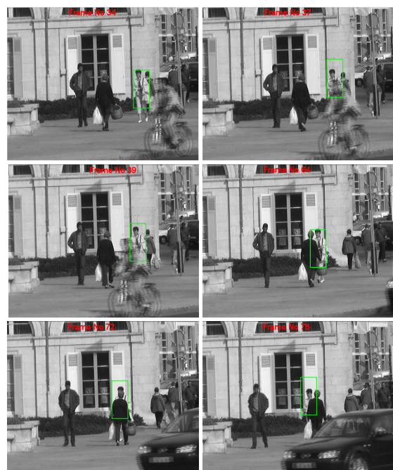
Figure 9 – Example of target tracking success with our algorithm on the OC1 sequence.
