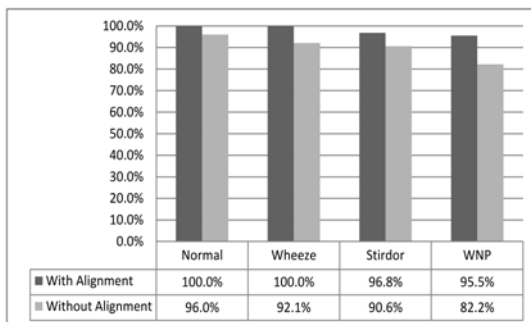
Figure 3: Performance of the proposed phase identification method with and without alignment scheme for MI calculation.
