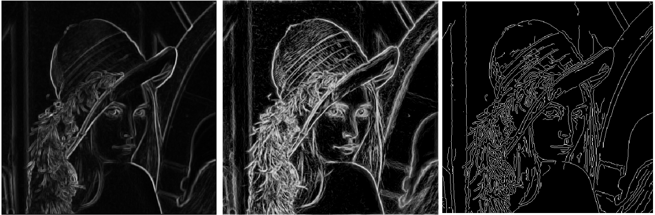
Figure 7: Edge detection in a real image using (from left to right): Error RMS, PC, Canny method.
