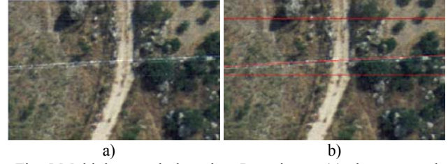
Fig. 5 Multiple scratch detection. Input image (a), three correctly detected scratches (b). Some scratches are not detected probably since “covered” by close ones.
