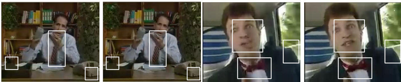
(a) 122 nd in "salesman" at 48Kbps (b) 186 th in "carphone" at 36Kbps Figure 6: Comparison of reconstructed frames with rate control in JM13.2 (Left) and with proposed scheme (Right).
