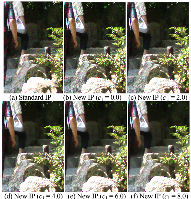
Figure 6 – Portions of color images restored from noisy mosaicked-color-data by the standard IP-pipeline and our new IP-pipeline in which the parameter c_1 is varied.
