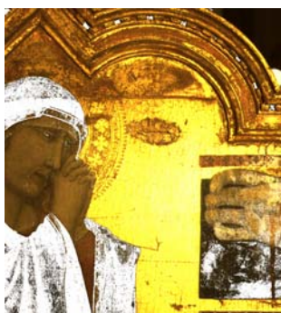
Fig. 10: attempt to identify pigments by using the spectral profile of its reflectance, using only 7 sub-bands in the visible range.
