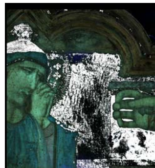
Fig. 9: attempt to identify a pigment by using the spectral profile of its fluorescence emission., using 7 images. A binary mask is superimposed to the fluorescence image
