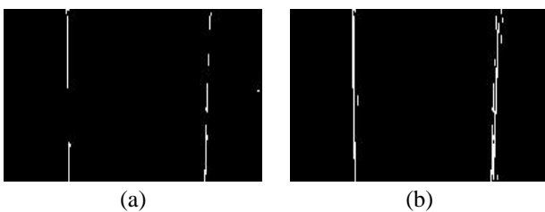
Figure 5: a) Broken segments after VA computation b) Segments reconnected after applying LC algorithm to connect lines.
