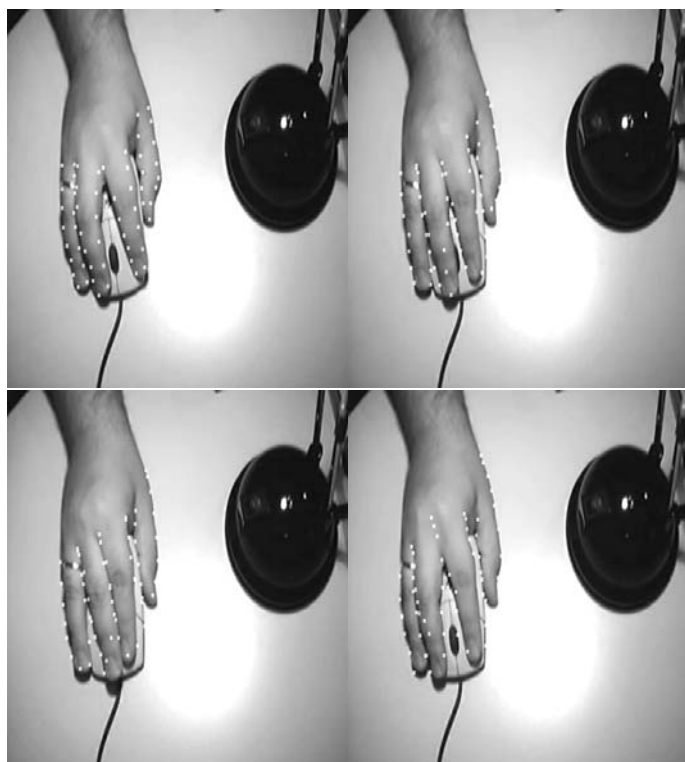
Figure 5: Finger tracking sequence obtained in the lab – Kullback-Leibler based tracking refinement scheme
