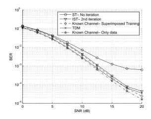
**Fig. 3**. BER for IST. '*Known channel-only data*': BER when the channel is completely known and full power is given to data; '*Known channel superimposed training*': BER when the channel is completely known and some of the data power is allocated for training.
