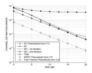
**Fig. 1**. Channel estimation error for IST. Note that IST approaches DDST. '*Fully trained*': all transmitted power used for channel estimation (benchmark for any trained algorithm). Note that TDM and DDST coincide and so are indistinguishable on graph.
