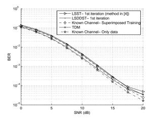
**Fig. 4.** BER for LSST and LSDDST. '*Known channel-only data*': BER when the channel is completely known and full power is given to data; '*Known channel superimposed training*': BER when the channel is completely known and some of the data power is allocated for training.
