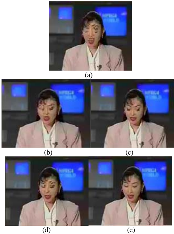
Figure 8. Effect of BEP TCH72(-85) on Akiyo sequence (a); simple ROI redundancy x2 and x3 (b-c); Interleaved ROI redundancy x2 and x3 (d-e).
