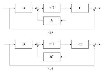
Figure 3: A realization of the conventional filterbanks (a) $\mathbf{E}'(z)$  (b) $\mathbf{R}'(z)$
