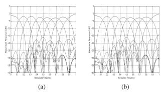
Figure 8: Frequency responses of 8-channel order-2 prop. FB: (a) analysis bank (b) synthesis bank
