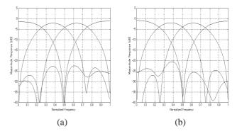
Figure 6: Frequency responses of 4-channel order-2 prop. FB: (a) analysis bank (b) synthesis bank.
