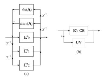
Figure 5: The structure of IIR-FIR hybrid building blocks: (a) analysis filter (b) synthesis filter.
