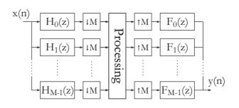
Figure 1: An M-channel filterbank.
