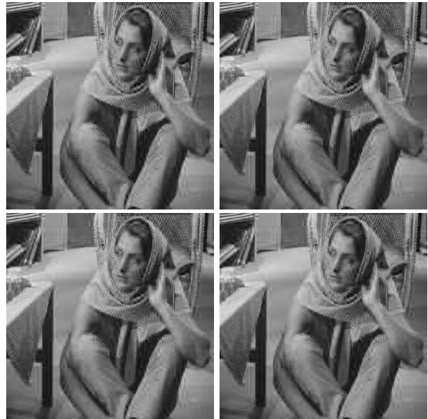
Figure 5: "Barbara" reconstructed from 2 levels of LP with 9/7 biorthogonal filters. top: (left) standard reconstruction (1.99 bpp, 29.96 dB), (right) frame-based reconstruction (1.99 bpp, 30.15 dB); bottom: (left) proposed method (1.62 bpp, 29.82 dB), (right) proposed method (1.99 bpp, 30.33 dB).
