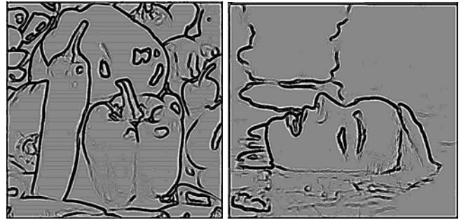
Fig.1. Map image \mathbf{M}(\mathbf{s}) shows the mean shift convergence frequency at each pixel position. (white: indicate edges, black: indicate nearer to edges; gray: indicate smooth areas. Left: from image “peppers”, right: from “swimming lady”).
