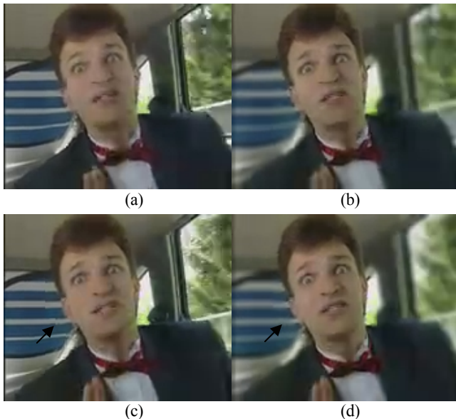
Figure 6 – Frame 64 of the compressed carphone sequence for 10 fps and 32 kbps with (a) no prefiltering, (b) spatial filter only, (c) temporal filter only and (d) spatio-temporal filter. The visual quality within the facial region is improved by using the spatio-temporal filter. In the temporally filtered cases (c,d) the trees outside the car window are positioned as in the previous frame. At the ROI border (see arrows) still some artefacts in (c) due to the large movement of the head in, but these are reduced in (d).
