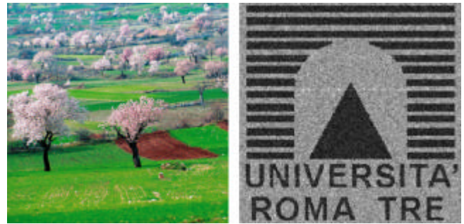
Figure 8 - (a) Image marked with “ROMA TRE” logo. (b) Extracted watermarking in presence of a loss of equal data to 6 bits on 512. (coefficient of correlation 0.90 – without loss of data the coefficient of correlation is 0.96)
