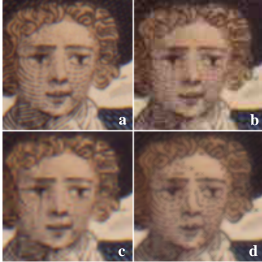
Figure 7. (a) Original image, (b) JPEG compressed, (c) JPEG2000 compressed and (d) MRC compressed image. Images are compressed at 40:1 compression ratio.
