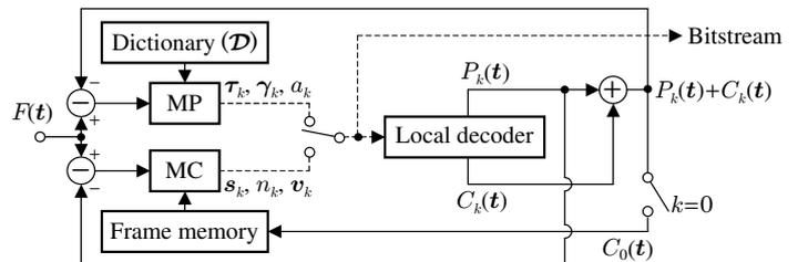
Figure 2: Block diagram of the encoder.
