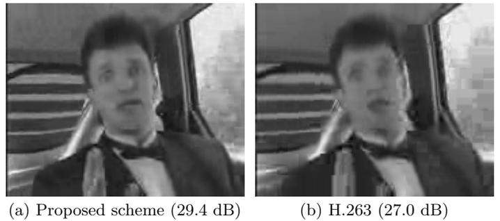
Figure 5: Examples of reconstructed images of ‘Carphone’ at 24 kbps of CBR coding (frame no. = 250).
