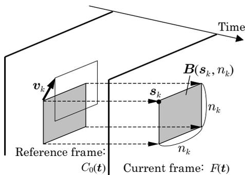
Figure 1: Iterative motion compensation method.
