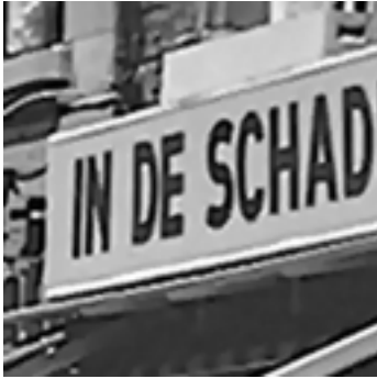
(b) Sharpened image by the thin-plate-deflection based method of the parameter setting of (\lambda, s, \sigma, K) = (1.0, 0.5, 1.0, 5.0) [ SNR = 22.882[dB], C_{\theta} = 0.112, Br = 0.513 , Nr = 0.136 ]
