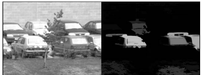
Figure 6. Left panel, V from Figure 1. Right panel, area sieved to keep just those local extrema of areas between 1000 and 4000 pixels.
