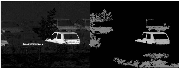
Figure 8. Left panel, H from Figure 1 that has been rotated before taking the cosine to emphasise reds. Right panel, the result of taking just the maxima of scales 1000 to 4000 pixels obtained from an area opening decomposition.
