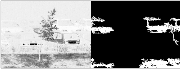
Figure 7. Left panel, H from Figure 1 that has been rotated before taking the cosine to emphasise blues. Right panel, the result of taking just the maxima of scales 1000 to 4000 pixels obtained from an area opening decomposition.
