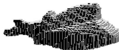
Figure 4.- Fish reconstruction with three views. Centroid is at x = 18.5 cm, y = -2.7 cm and z = 153.9 cm in sonar co-ordinate system. Positioning angles are \theta = -6.1^\circ , \phi = -3.5^\circ and \psi = 3.3^\circ .
