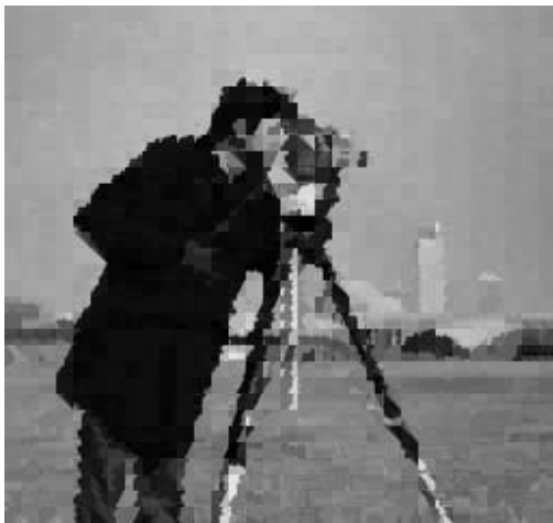
Figure 4: “Camera,” Mixed Algorithm: PSNR_{L_2} = 21.94 dB, PSNR_{L_1} = 28.62 dB, bit rate = 0.27 bit per pixel.
