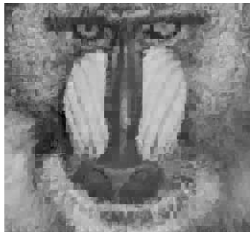
Figure 7: “Ape,” L_1 Algorithm: PSNR_{L_2} = 18.50 dB, PSNR_{L_1} = 21.63 dB, bit rate = 0.27 bit per pixel.
