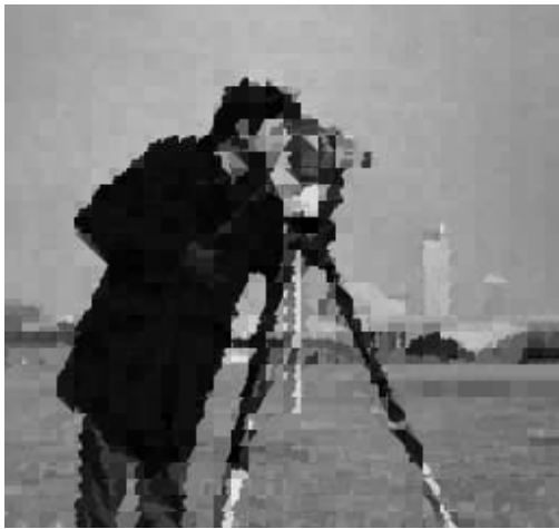
Figure 3: “Camera,” L_1 Algorithm: PSNR_{L_2} = 21.98 dB, PSNR_{L_1} = 28.62 dB, bit rate = 0.27 bit per pixel.
